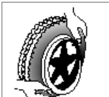
Push the tyre over the edge of the rim, starting behind the air valve. Inflate the tube slightly until it is round, and place it inside the tyre.
